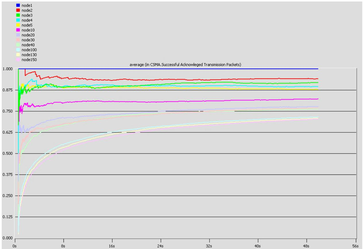
Figure 5: Average successful acknowledged transmission packets for different numbers of end nodes.
