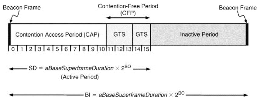
Figure 1: Frame structure of the beacon signal [10].
