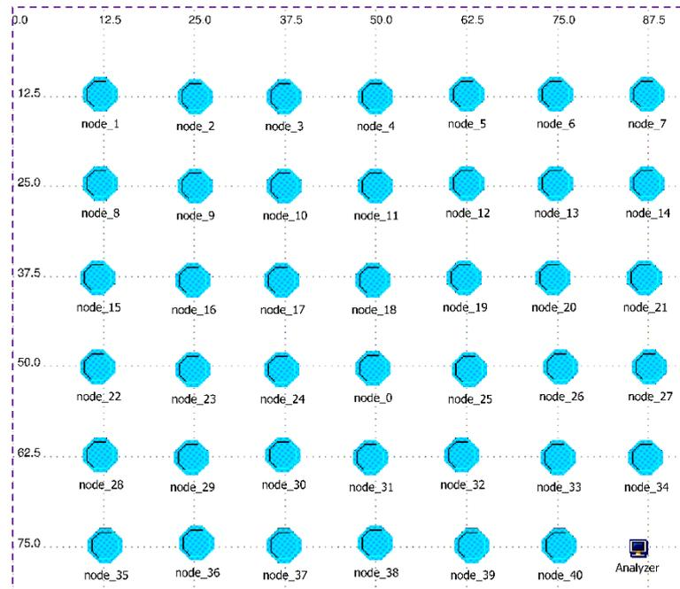
Figure 3: Example of star topology with 40 ZigBee end-nodes inside 100m<sup>2</sup> room.
