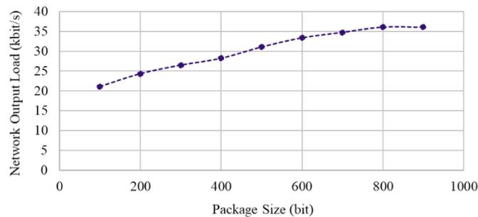
Figure 7: Network output load as a function of packet size.
