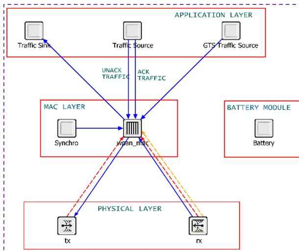
Figure 2a: IEEE802.15.4 OPNET simulation model.
