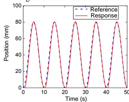
Figure 7: Comparison between the reference and the actual position of the mass
