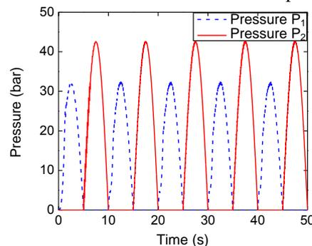
Figure 9: The pressure state of the ports of the hydraulic
