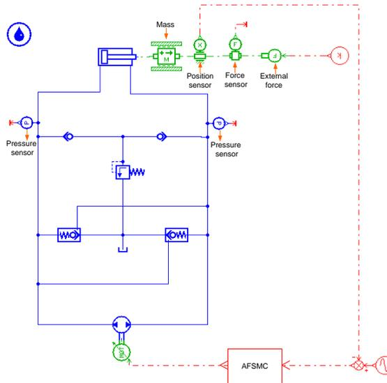
Figure 4: The virtual model of EHA by using Amesim software
