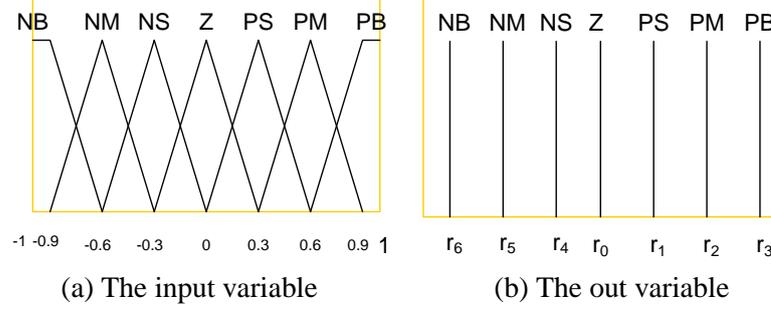
Figure 3: The membership functions for the input variable  $s$  and the output variable  $u_{hit}$
