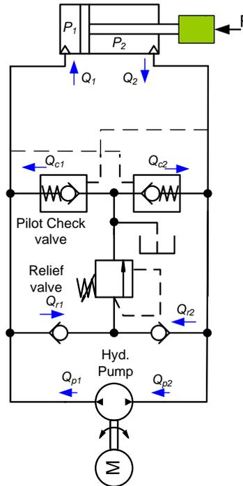
Figure 1: Schematic diagram of an electro-hydraulic actuator
