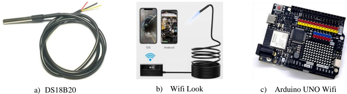
Figure 6. Illustration of a) Temperature sensor, b) Endoscope Wi-Fi camera and c) MCU.
