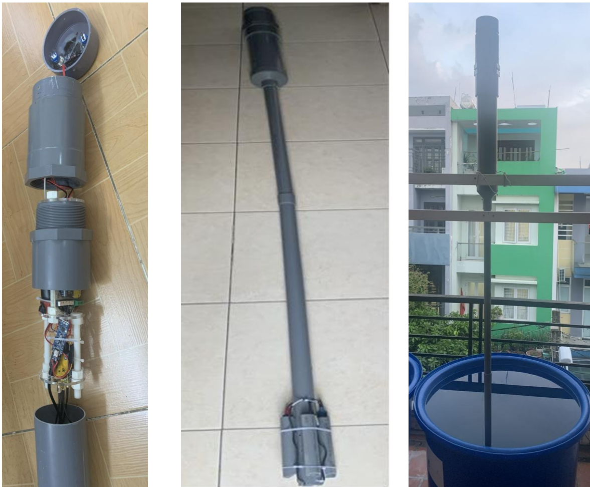
a) Installation of component modules.
