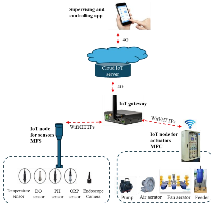
Figure 14. Illustration of the integration of MFS into the MFC automation control system for HTSF.
